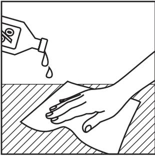
**1** Make sure the surface on which the LED tape is to be applied is flat, smooth, dry and clean.
